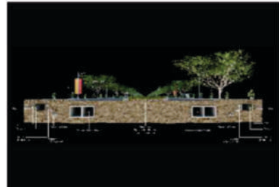
Utility Corridor Underground Utility Network for Water, Power, Gas, ICT and Waste Water Collection
